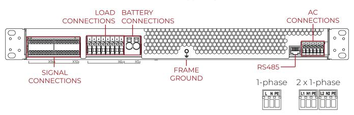
Note that when the 1-phase configuration is selected only the left hand set of 3 terminals is present and this is connect to both rectifier positions within the unit.
