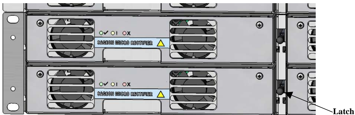
FIGURE 6-2 REMOVING RECTIFIER MODULE
